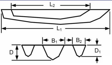
the face of the bow or stem aft to the top of the transom at the deck—don't include bowsprits, boarding steps, motor brackets, pulpits, etc. Depth of hull is the vertical height from the deck at side down to the top of the keel taken at midships—it is *NOT* draft. (See illustration above.)
